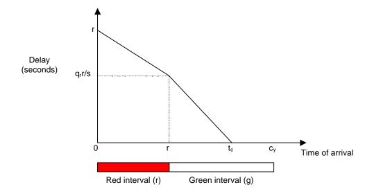
Figure 3: Uniform queue delay as a function of vehicle arrival time
