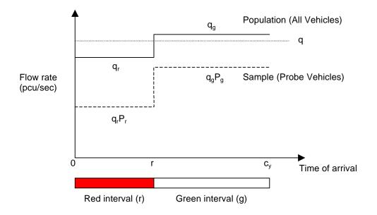
Figure 1: Illustration of arrival rates for probe vehicles and all vehicles during the red and green intervals
